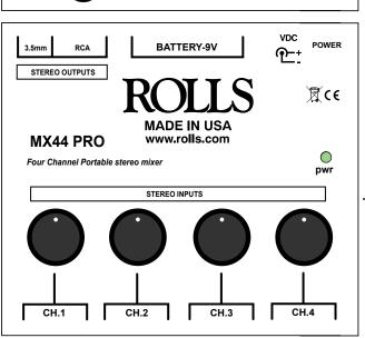
OUTPUTS: 1/4" and 1/8" (3.5 mm)Tip-Ring-Sleeve jack for connection to a mixer input, amplifier or other input device.
